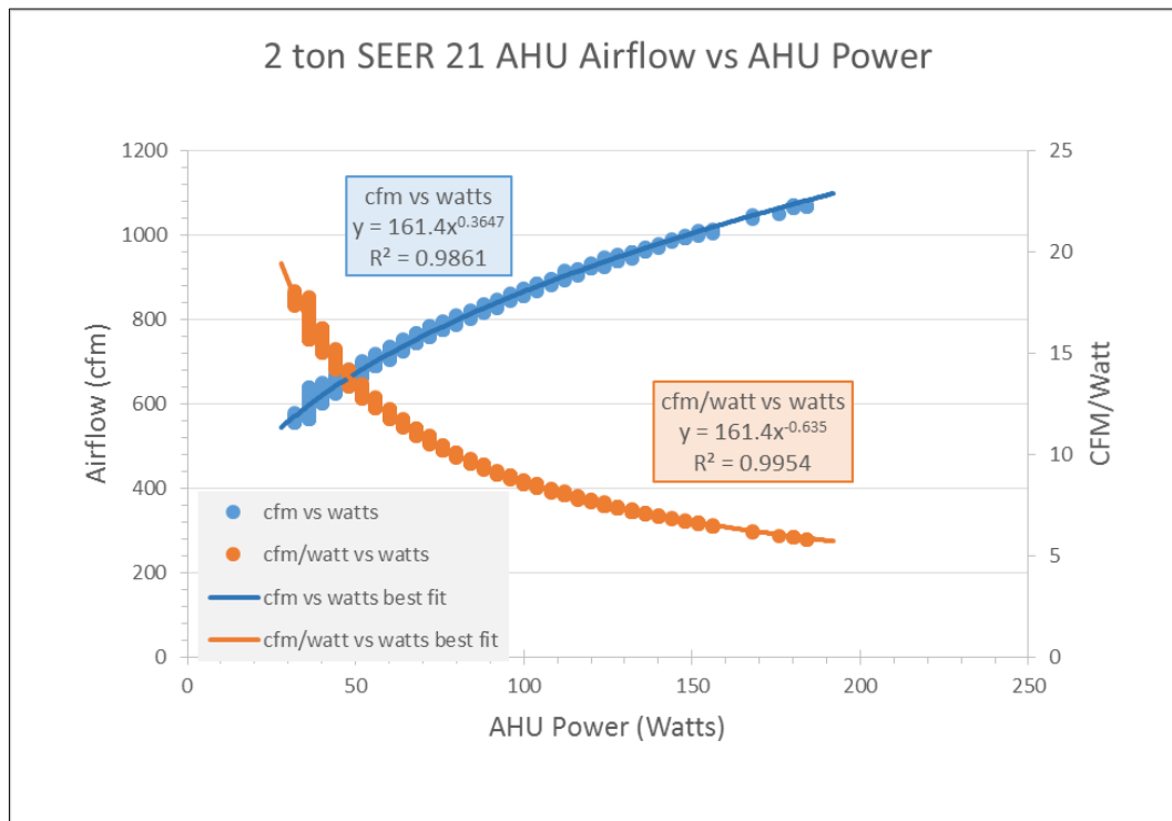
Figure 1. SEER 22 2-ton heat pump AHU fan power consumption measured in the lab
