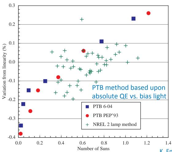
PTB method is the most correct procedure because it relies on the change Jsc from the absolute QE vs. bias light.
