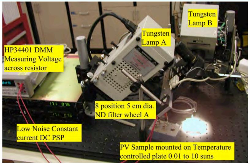
Linearity test bed to demonstrate that Isc is linear with irradiance as required in reference cell calibration and IV measurement standards.
