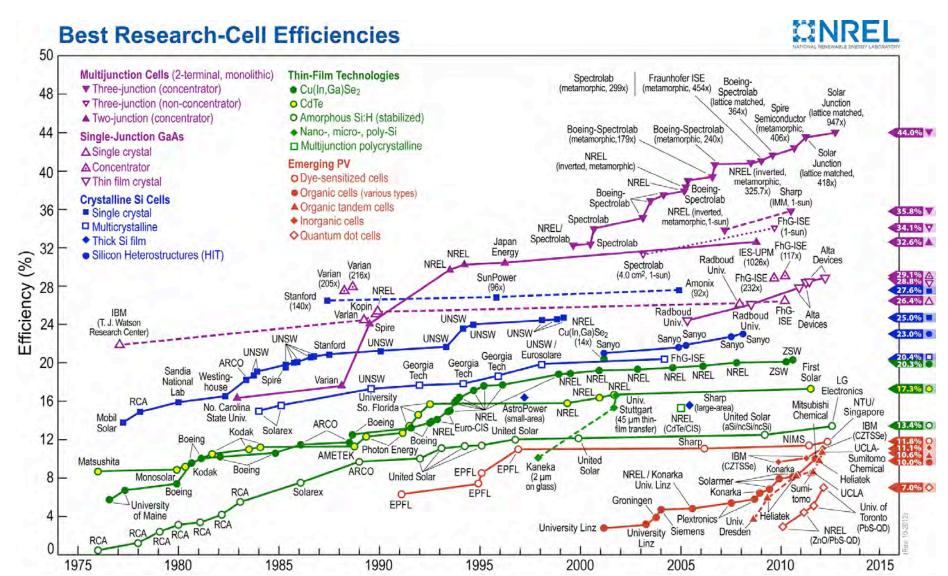
Record cell efficiencies over time by technology measured by recognized independent test labs.
