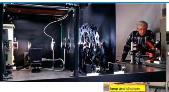
The spectral responsivity is measured with a filter based system (280-1800 nm) or a grating based system 350-2800 nm
