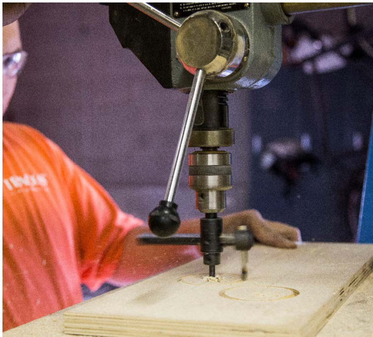
Figure 3. Using an adjustable-hole saw to cut the manifold outlets
