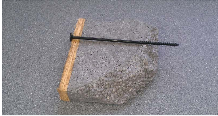
Figure 5. SIP screw and piece of 6-in. graphite-enhanced EPS nail base panel
