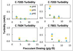
All flocculants showed significant reduction in turbidity from a baseline hydrolyzate turbidity of 1.288 mAU. Due to the low dosing of flocculant necessary to yield low values of turbidity and total solids, KemSep C-7205 was selected for further testing with an expanded range of loadings and pH values.
