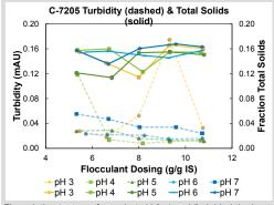
Flocculation tests performed at pH 3, 4 and 5 yielded the best results, as shown above. Increases in total solids around flocculant dosings of 7-8 g/g-insoluble-solids are thought to result from excess flocculant present in the extracted liquor, with the lowest total solids values showing an approximate optimum flocculant loading.
