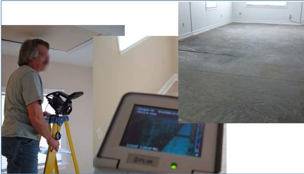
Figure 20. Setup for time lapse thermography of uncovered west building slab floor on the coldest night of 2013
