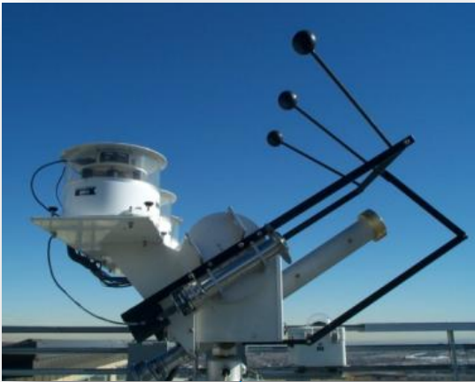
Reference Diffuse Traceable through Cavity using Shade/Unshade method
