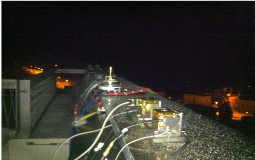
ACP & IRIS nighttime comparisons at PMOD; difference is within 2 \text{ Wm}^{-2} in two comparisons
