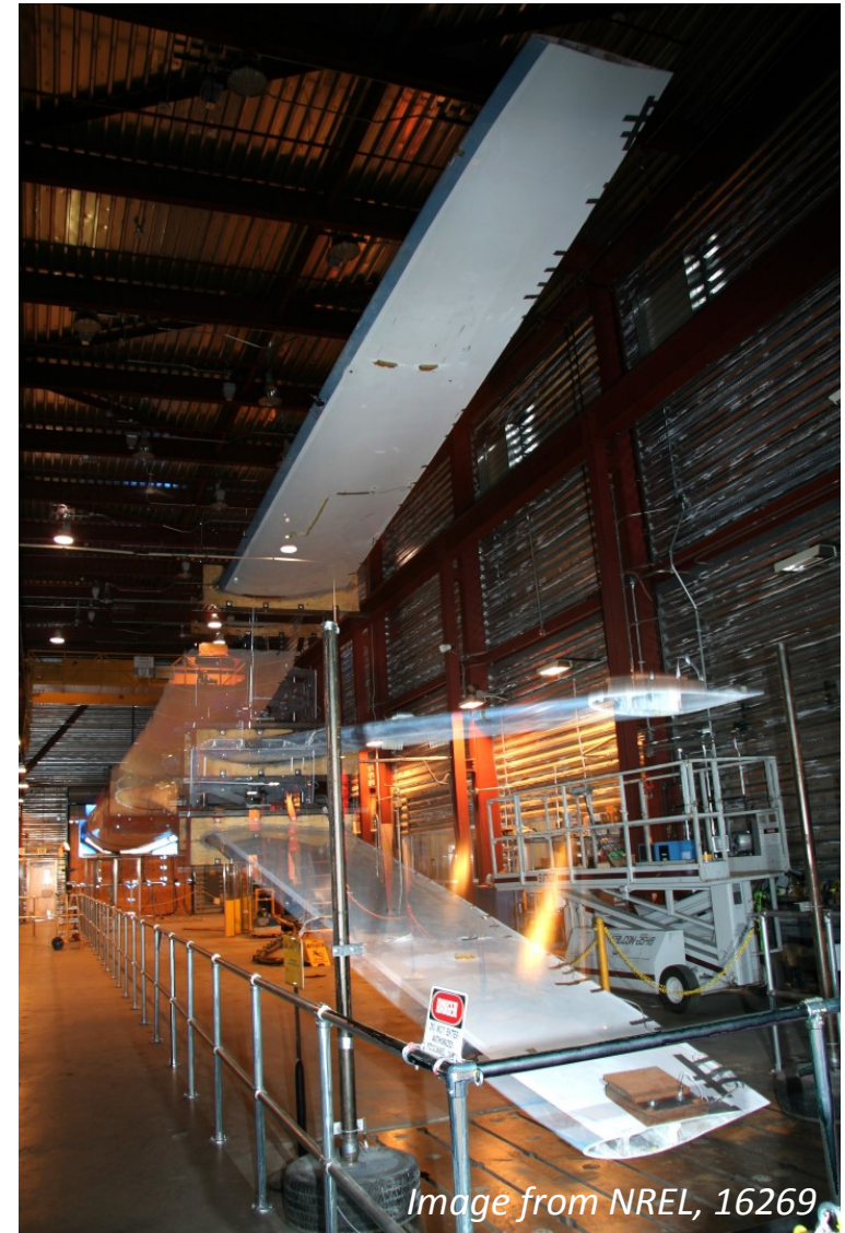
Inertial mass flap fatigue test at National Wind Technology Center, Boulder, CO
