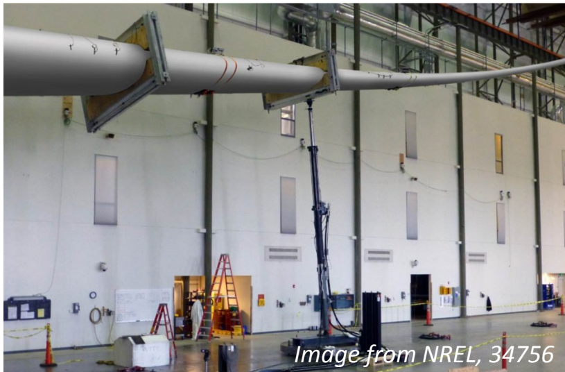
Flap fatigue test at Wind Technology Testing Center, Boston, MA
