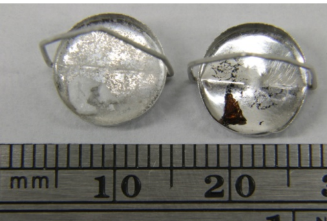
Representative photo of residual char from specimens tested in an O 2 -containing or N 2 -only atmosphere.
