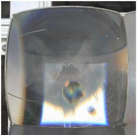
10 cm 1 of 5 lens sites damaged (cracked) in a hail storm on 2010/6/11.
