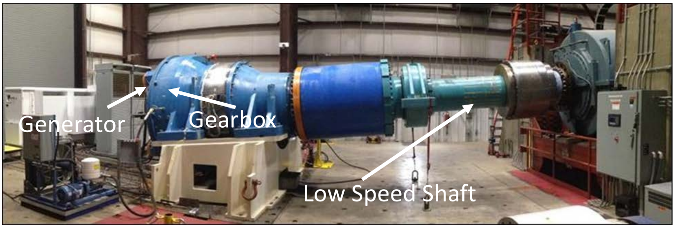
Fig. 2. Photograph of completed next-generation drivetrain during dynamometer testing. Photo by Jonathan Keller, NREL 35206
