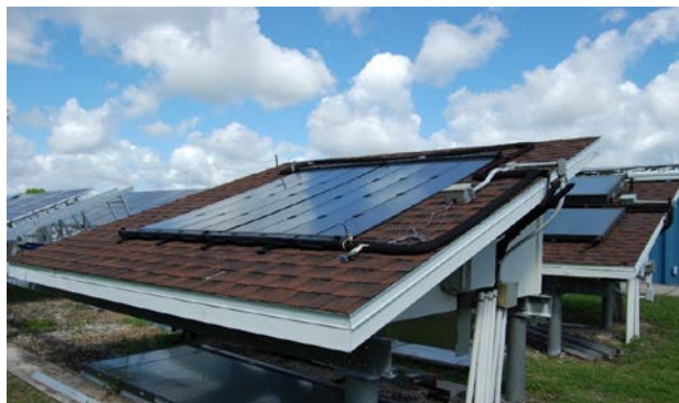
Figure 5. Solar polymer collector (glazed) at FSEC's HWS laboratory (Cocoa, Florida) mounted on roof test stand
