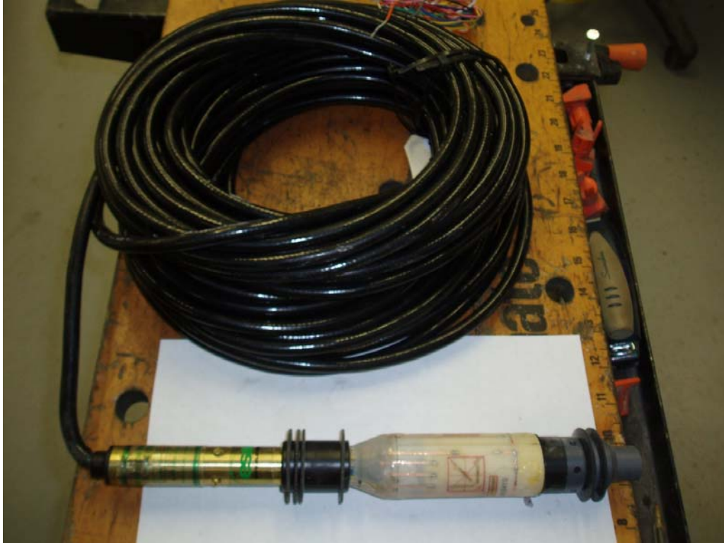
Figure 5. CSIRO HI Stress Cell with Cable Attached
