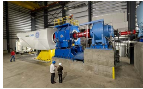
Figure 7. 2.75-MW WTG drivetrain under test
