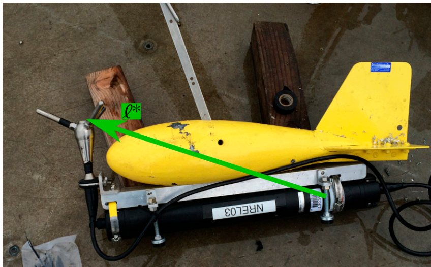
FIG. 5. The turbulence platform showing details of the ADV head and pressure case configuration. The green arrow indicates the vector from the IMU to the ADV head. The head cable was taped out of the way beneath the sounding-weight tail fins shortly after this photograph was taken.
