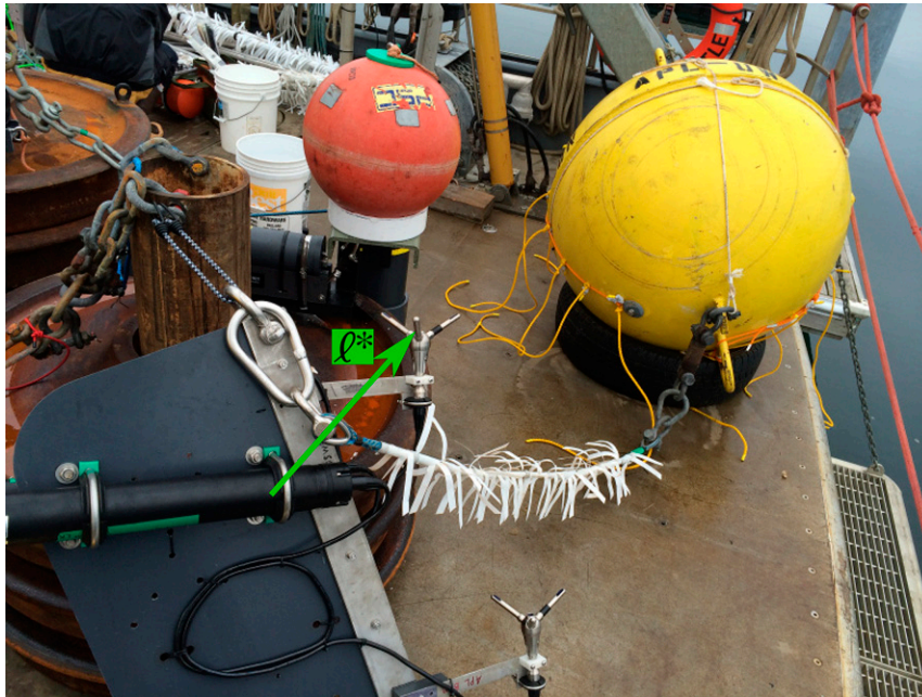
FIG. 3. TTM components on the deck of the R/V Jack Robertson . The TTM includes two ADVs, with pressure cases mounted on opposite sides of the fin. The anchor stack includes a pop-up buoy for retrieval. The green arrow indicates the vector from the IMU to the ADV head (face of the transmit transducer).
