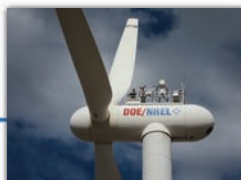
Impact detection testing on the three-bladed Controls Advanced Research Turbine. Photo by Lee Jay Fingersh, NREL 40948
