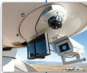
Visual, infrared, and thermal monitoring test from one turbine to a neighboring turbine at the NWTC. Photo by Lee Jay Fingersh, NREL 40949
