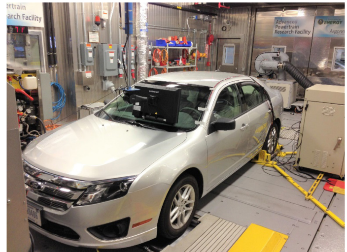
Figure 5. 2011 Ford Fusion test vehicle on Argonne’s APRF dynamometer for testing.
