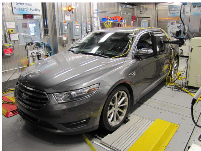
Figure 3. 2013 Ford Taurus on Argonne’s APRF dynamometer for testing.
