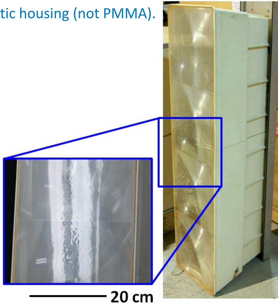
Photographs of M-M module (NREL warehouse), revealing the dimpled surface of the lens.
