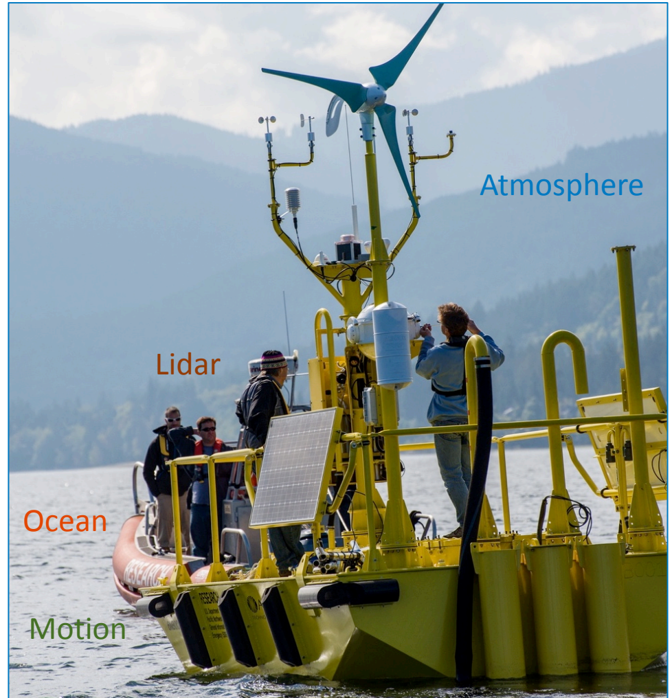
AXYS FLiDAR 6-meter (m) buoy. Photo from Flickr, courtesy of Pacific Northwest National Laboratory
