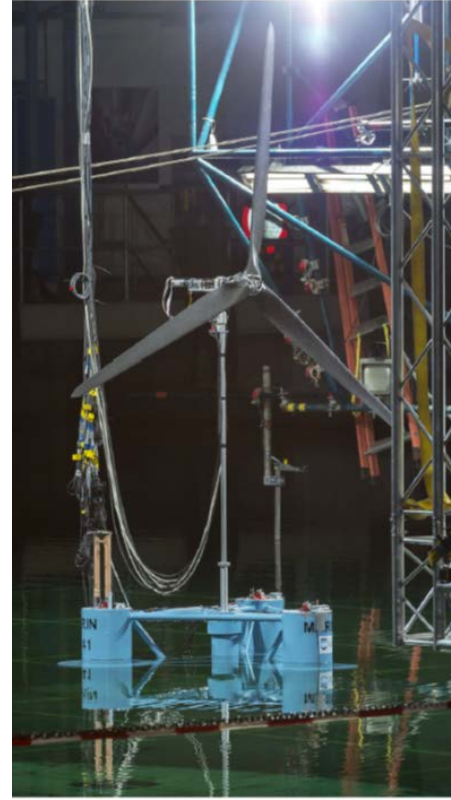
Fig. 1. Instrumented OC5-DeepCwind model in the MARIN offshore basin (Helder and Pietersma, 2013)
