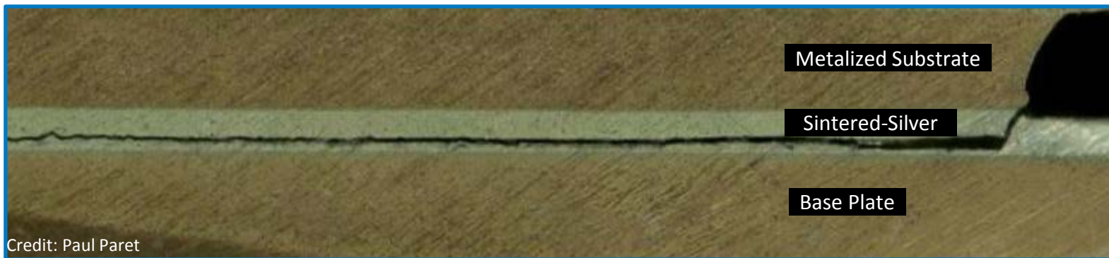
Crack Propagation in Sintered-Silver
