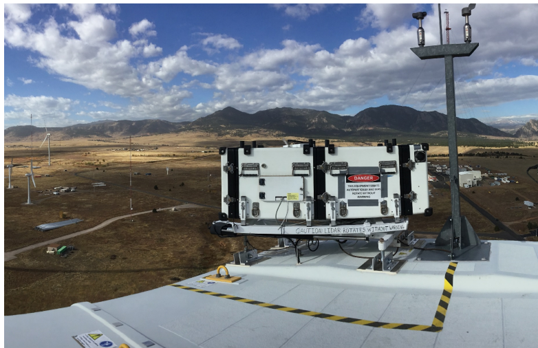
Figure 2: The University of Stuttgart lidar installed on the DOE 1.5 turbine. Photo by Andrew Scholbrock, NREL
