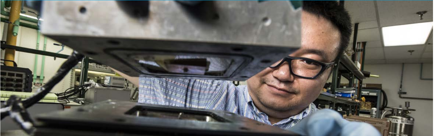
A researcher prepares the Micro Calorimeter for coin cell battery evaluation. The unique busbar design allows for the assessment of battery cells under load. Photo by Dennis Schroeder, NREL 44055
