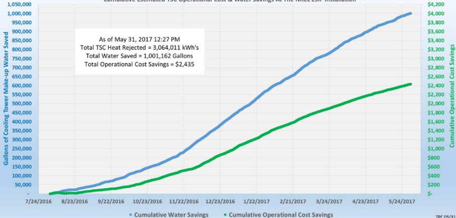
Cumulative Estimated TSC Operational Cost & Water Savings At The NREL ESIF Installation
