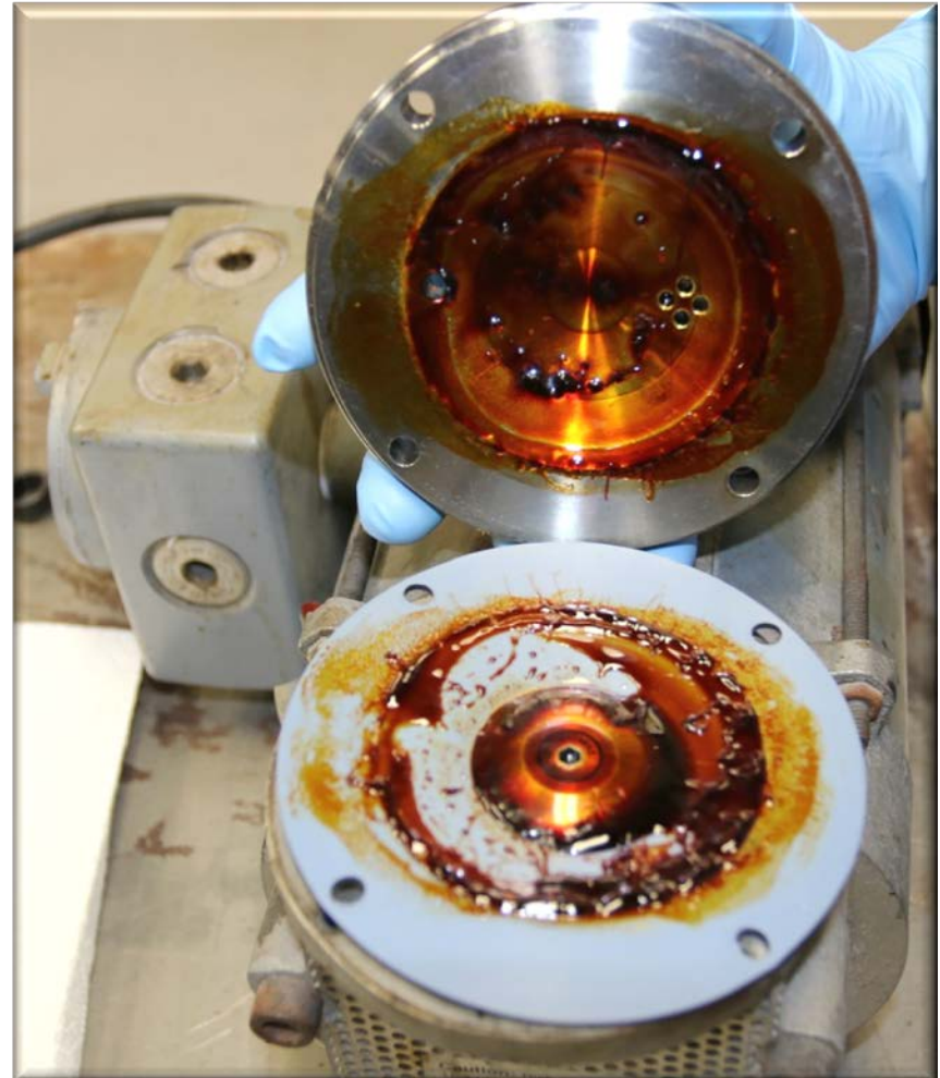
Pyrolysis buildup in pump head – located after a condenser and coalescing filter
