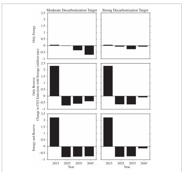
Figure 5. Change in system  $CO_2$  emissions with storage versus without storage under the moderate (left) and strong (right) decarbonization targets when storage participates in only energy (top row), only reserve (middle row), or energy and reserve (bottom row) markets. Positive values indicate storage increases  $CO_2$  emissions.
