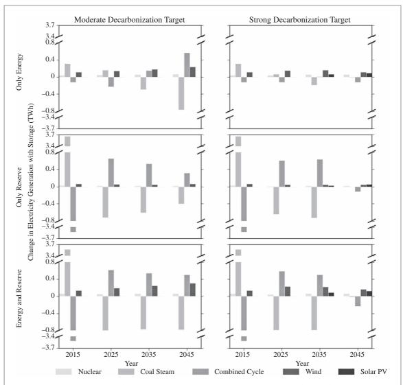
Figure 4. Change in generation by fuel type with storage versus without storage under the moderate (left) and strong (right) decarbonization targets when storage participates in only energy (top row), only reserve (middle row), or energy and reserve (bottom row) markets. Positive values indicate storage increases generation.
