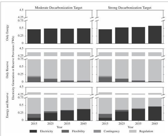
Figure 2. Storage electricity generation or flexibility, contingency, or regulation reserve provision under the moderate (left) and strong (right) decarbonization targets when storage participates in only energy (top row), only reserve (middle row), or energy and reserve (bottom row) markets.
