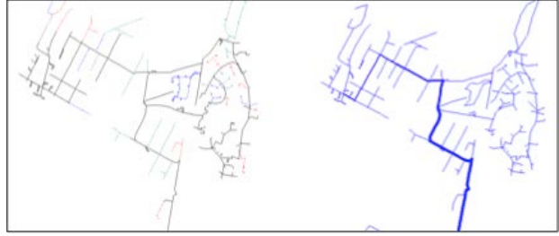
Figure 1. Geographical view of L distribution feeder in the commercial distribution software on the left and OpenDSS on the right.
