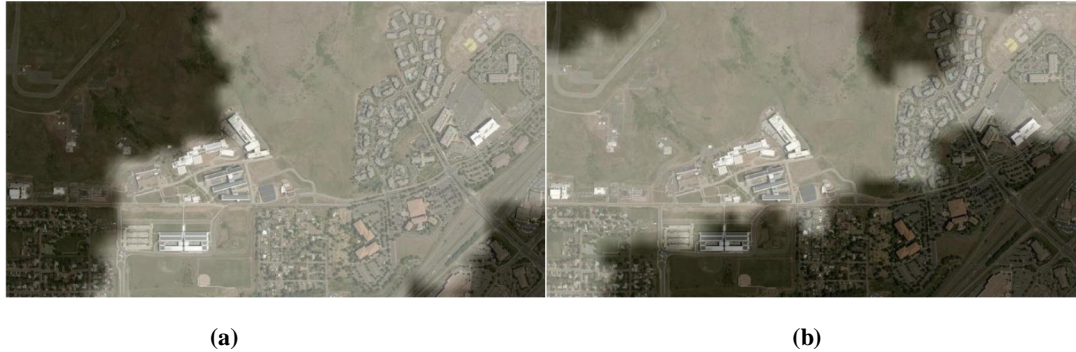
Figure 52: (a) Current cloud cover at NREL; and (b) cloud cover over NREL 5-min ahead. Note: clear sky appears bright and shading appears black
