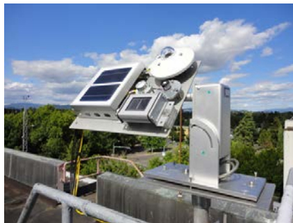
Fig. 1: Pyranometers and reference cells on a one-axis tracker in Eugene, Oregon.
