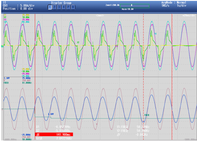
Fig. 3. Oscilloscope screenshot showing time series waveform results for Test Case #3. The top plot shows current meas. for each deferrable load including the fridge (“I1”, yellow), bank of light bulbs (“I2”, green), plug-in heater (“I3”, purple), and oven (“I4”, cyan). The bottom plot shows the grid voltage (pink), calculated grid frequency (green), and inverter current (blue). It can be seen that the entire net-load response sequence is completed within 142 ms (~8.5 ac cycles).
