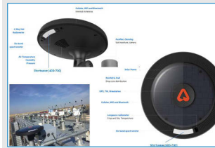
Fig. 1. Arable's Mark low-cost, multiparameter system at the NREL SRRL
