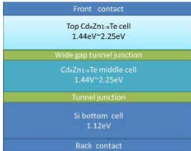
Fig. 8. Example CZT/Si-based multijunction device structure.
