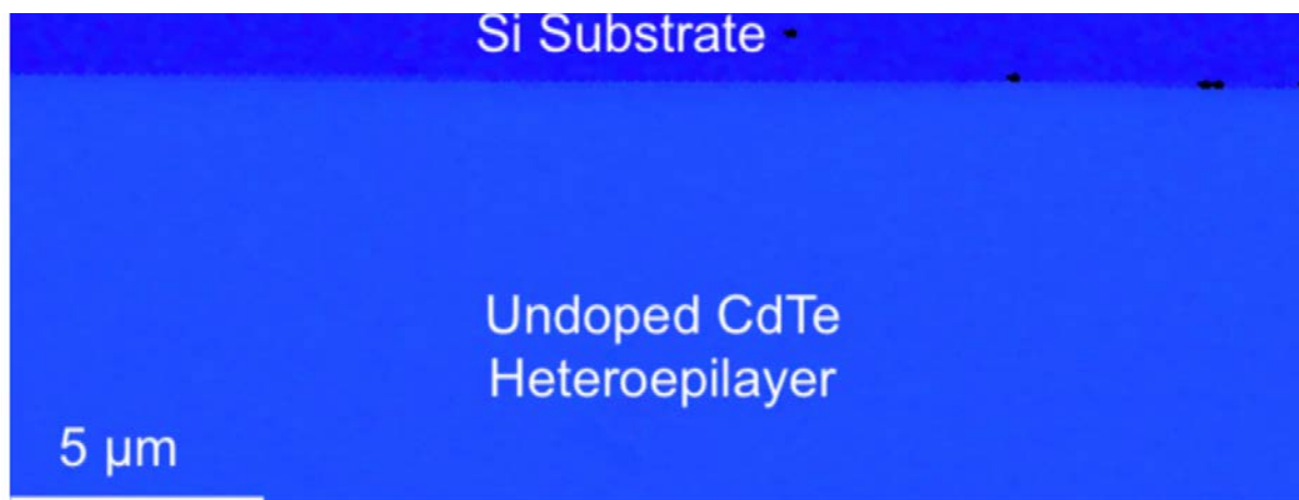
Fig. 7. Si/CdTe heterointerface region for MBE-grown undoped CdTe layer with 14% Te overpressure (sample w13042). Total undoped CdTe film thickness for this sample is 5.5 microns.
