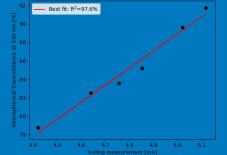
The results show that the two measurements have a R<sup>2</sup> of 97.6%, a strong linear correlation between the measurement of DUSST and the actual transmittance of the glasses at the same wavelength as the diode used in the prototype.
