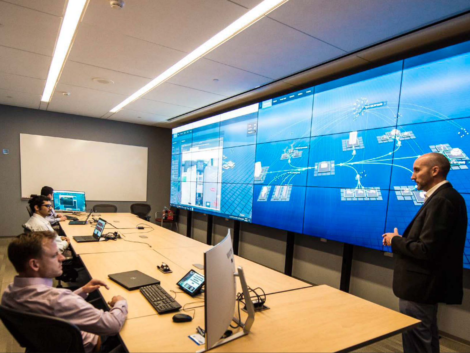
At the Energy Systems Integration Facility, NREL analysts can visualize a virtual grid environment with connections to both emulated and real physical devices in the facility and at NREL's Flatirons Campus.
