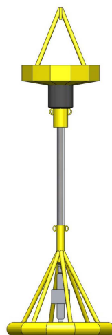
Figure 1. RM3 1:100-scale model [13].
