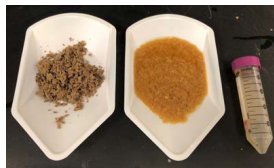
Figure 2. DMR pretreated corn stover (Left) versus DMR pretreated corn stover following treatment using Fenton reactions (Middle). Right: condensate collected after reaction.
