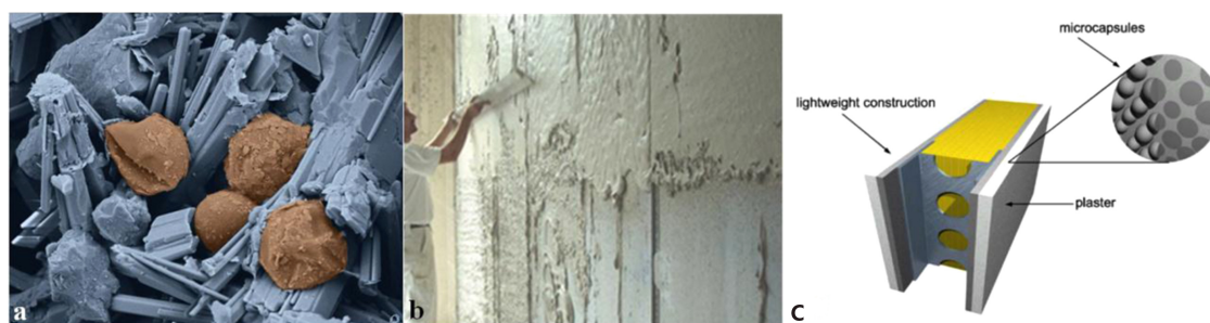
Figure 5. Examples of phase change materials (PCM) integration in envelope, adapted from Reference [14]. (a) Electron microscopy of PCM in gypsum plaster, (b) Wall finishing for gypsum plaster, (c) PCM micro-capsules.
