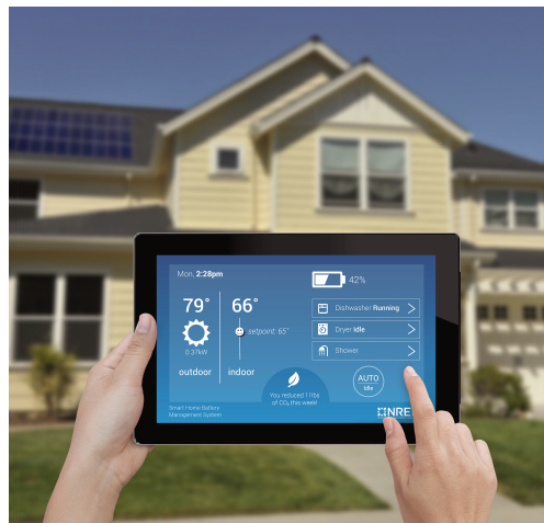
Figure 2. FORESEE is a home energy management system (HEMS) that allows homeowners to track energy use as well as balance, prioritize, and control end uses including lighting, space conditioning, water heating, and appliance usage. Images courtesy of the National Renewable Energy Laboratory (NREL).
