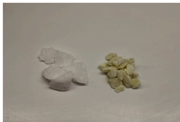
Fig. 6. Salt color for purified AC + halite (left) and as-received AC (right). (For interpretation of the references to color in this figure legend, the reader is referred to the Web version of this article.)
