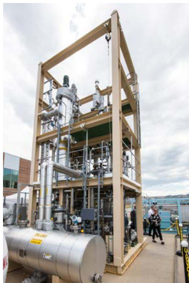
The Energy Systems Integration Facility's 700-L pressurized gas bioreactor designed for hydrogen and carbon dioxide gas feeds.
