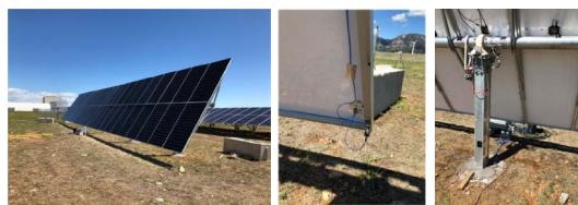
*(left) A solar PV tracker wind loading experimental setup showing instrumentation*
