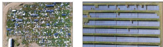
*Two images showing various impacts from the same storm in Puerto Rico. Humacao installation (left) suffered near total damage while Oriana array (right) needed replacement of only ~10% of modules, largely because of superior structural design*
