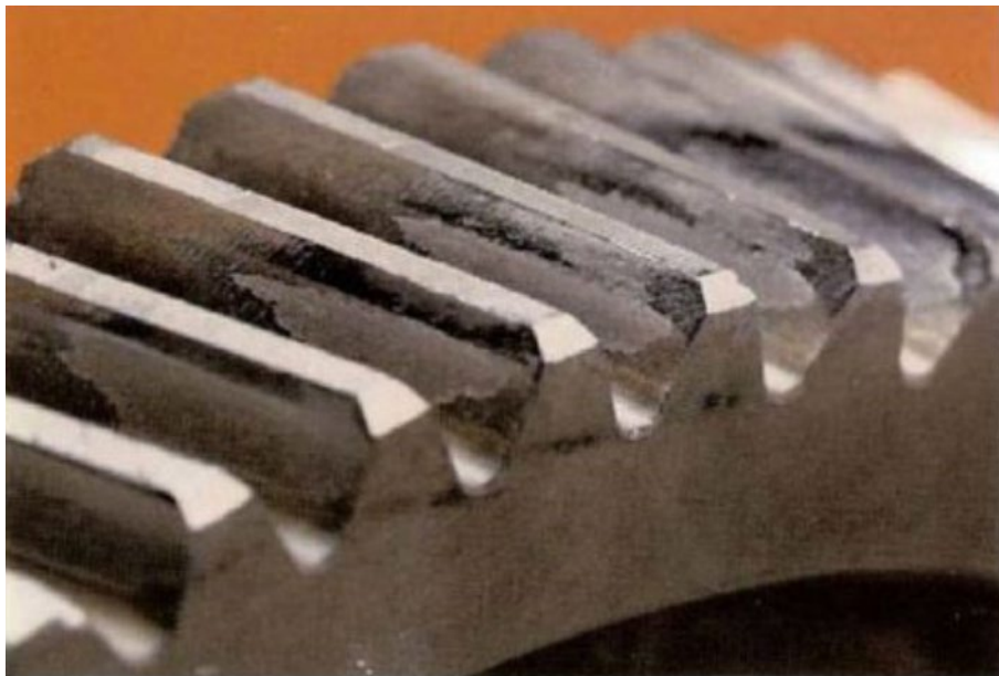
Figure 1 - Micropitting on a carburized gear (From ANSI/AGMA 1010-F14 [1])
