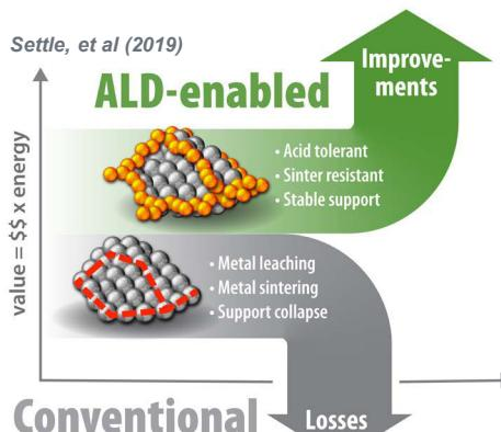
$TiO_2$  and  $Al_2O_3$  ALD overcoats applied to supported Pd catalysts for hydrogenation reactions
