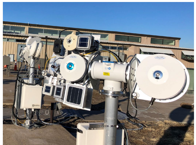
Fig. 1 Two-axis tracker and instruments at NREL. A one-axis tracker with similar instruments is in the background.
