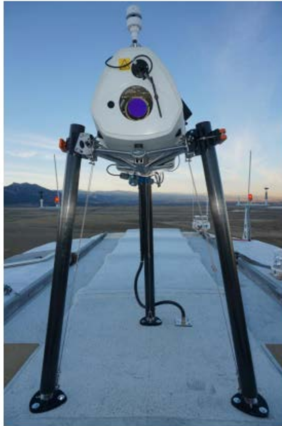
Figure 7. Lidar installed on nacelle roof of ECO110 wind turbine at NREL
