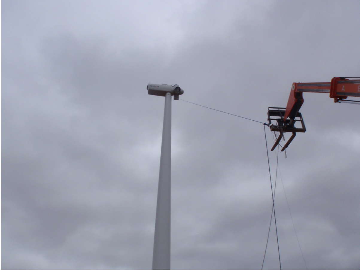
Figure 9. Snapback excitation on the ECO86 turbine in Lubbock
