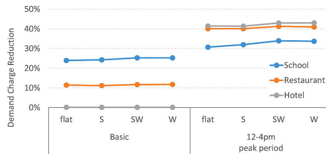
Fig. 15. Demand charge reductions across PV panel orientations for three commercial building types.
