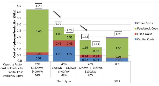
Availability of low-cost electricity can help enable *low*cost hydrogen production at *lower capacity* factors
