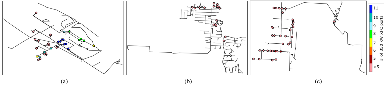
Fig. 6. Feeder circuit showing the nodes capable of hosting xFC EV load for (a) Feeder 1, (a) Feeder 2, and (a) Feeder 3.
