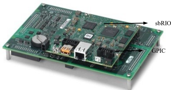
Fig. 9. Controller used in the CHIL setup.
