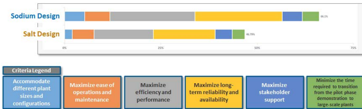
FIGURE 4. Benefit scoring results. Stacked bar chart (larger bar = higher benefit). The sodium receiver outscores salt on all benefit criteria.
