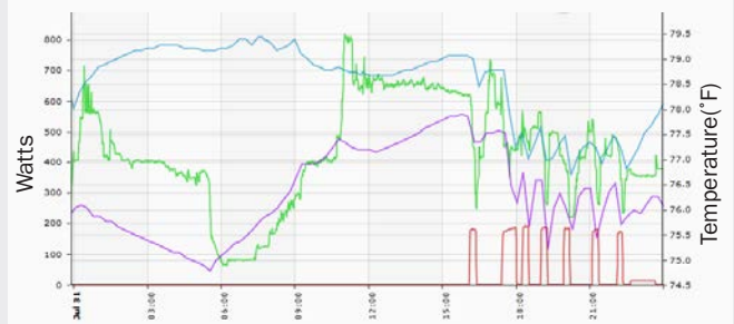
Figure ES-3. MSHP and CSCS energy profile under integrated control: CSCS power/10 (red), MSHP power (green), living room temperature (purple), master bedroom temperature (light blue)
