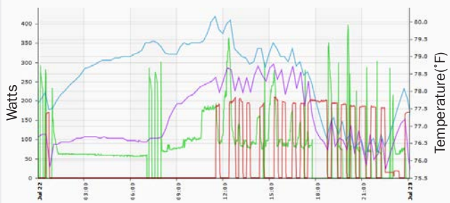
Figure ES-2. MSHP and CSCS energy profile under manual control: CSCS power/10 (red), MSHP power (green), living room temperature (purple), master bedroom temperature (light blue)
